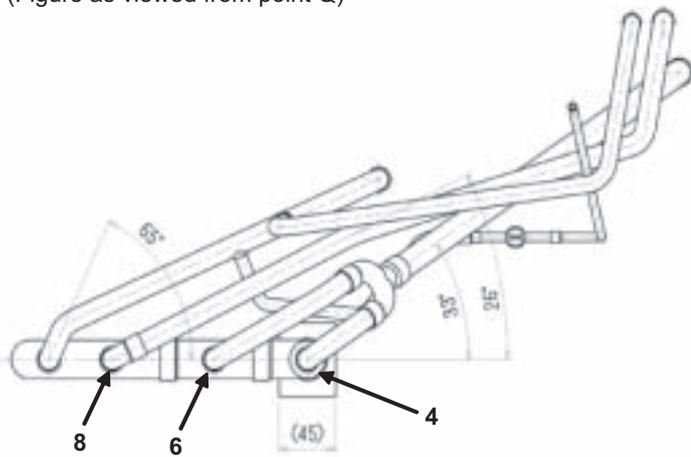
**2. Solenoid valve block ASSY (SV4a, SV4b, SV4c, SV4d), Check valve (CV4a, CV6a, CV8a, CV9a, CV10a) replacement instructions**
