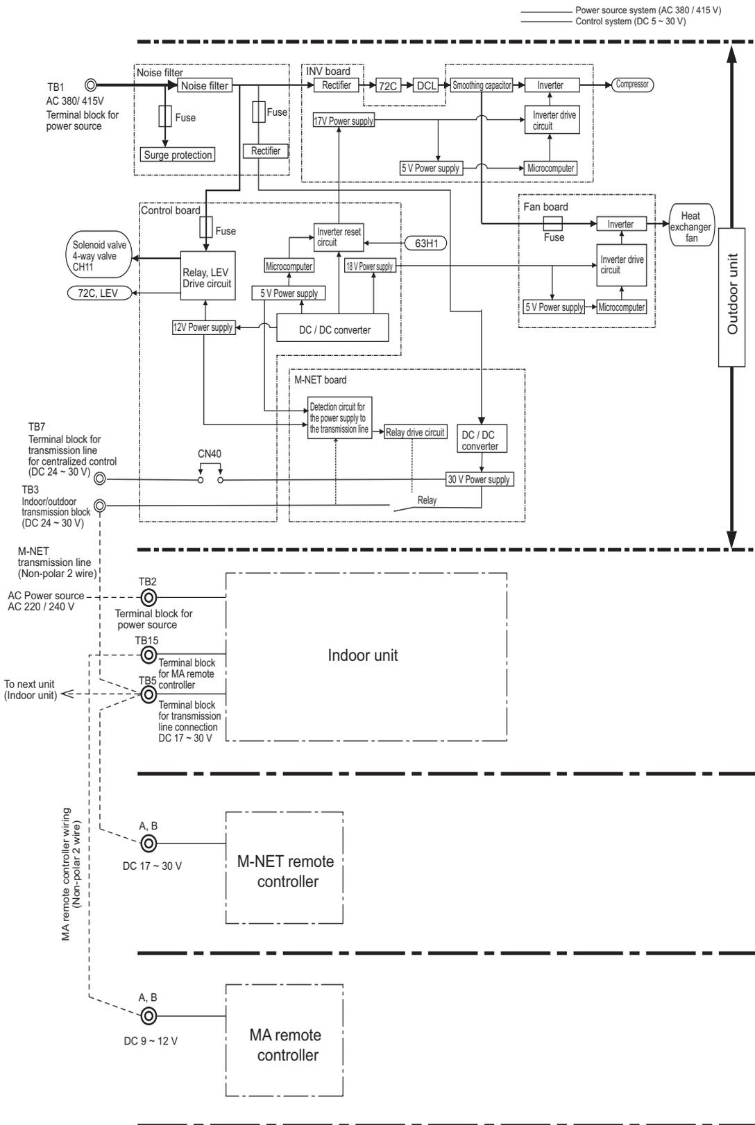
\* MA remote controllers and M-NET remote controllers cannot be used together.
