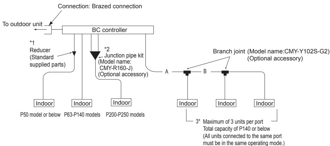
The ports of the BC controller accommodates the pipes on P63-P140 models of indoor units. To connect other types of indoor units, follow the procedure below.
