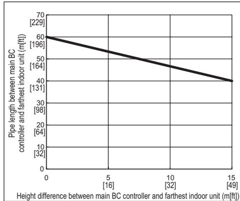
**(2) System that requires more than 16 BC controller ports or with multiple BC controllers <Outdoor unit (E)P400 model or below.>**
