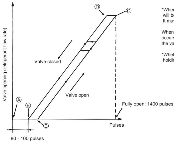
\*When the power is turned on, the valve closing signal of 2200 pulses will be output from the indoor board to LEV to fix the valve position. It must be fixed at point (A)
