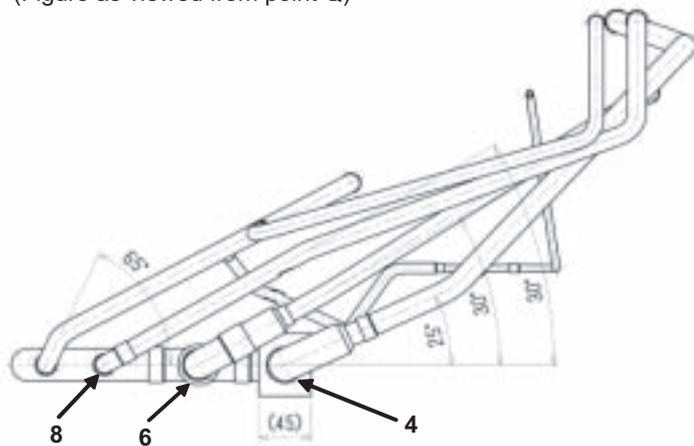
**3. Solenoid valve (SV1a), Capillary tube ASSY (CP1) replacement instructions**
