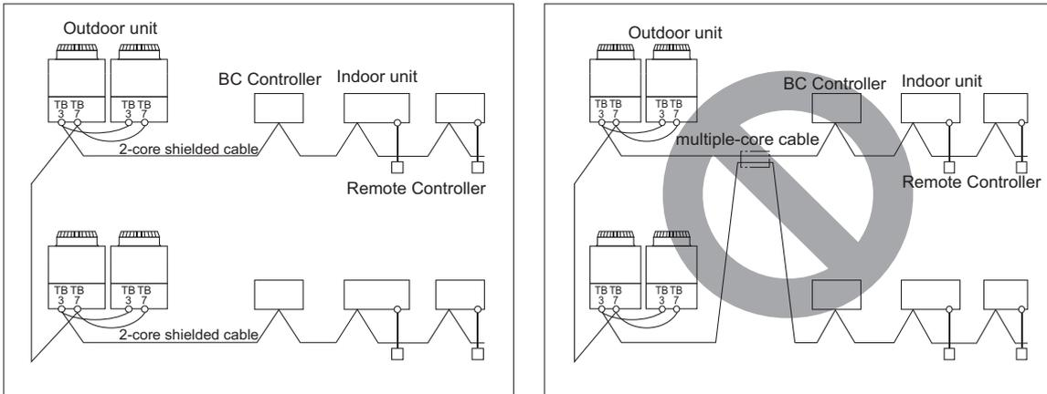
TB3: Terminal block for indoor-outdoor transmission line TB7: Terminal block for centralized control
