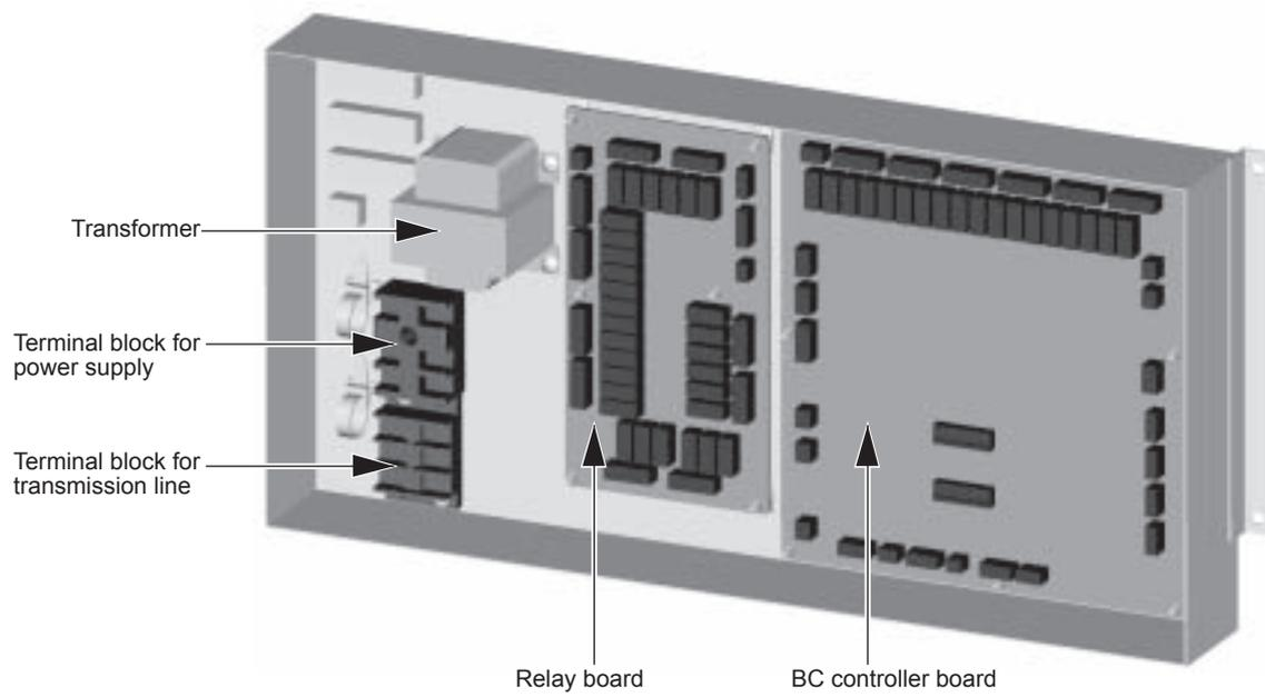
2. RELAY BOARD (RELAY 4 board)
